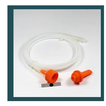
The ParaSure Single Lumen Channel Control 1 (SLCC1) simulates fine lumen devices and endoscope channels with a 1mm internal diameter, to effectively test the washer-disinfector's performance. The polypropylene head houses the indicator and is connected to a 1.5 metre length of PTFE tubing which terminates in a luer lock.
