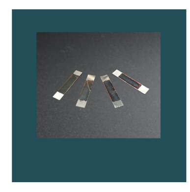
The ParaSure Synthetic Cleaning Efficacy Indicators offer a unique and cost-effective option for all healthcare facilities to ensure the decontamination process and soil removal efficacy is in accordance with EN ISO 15883 1-2-5. The indicators are designed to be used in conjunction with the ParaSure Standard Metal Basket (PS1610).
