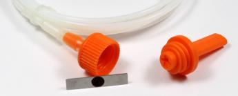
For monitoring the cleaning efficacy in flexible endoscopes to EN ISO 15883-5:2005
