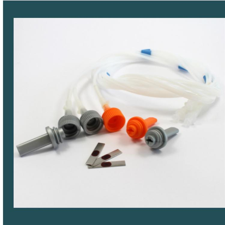
The ParaSure Multi Lumen Channel Control (MLCC) simulates an endoscope with 3 channels (1 x 1mm diameter and 2 x 2mm diameter), providing a unique solution to realistically test the effectiveness of the washer-disinfector. The MLCC combines 3 polypropylene head indicator holders, each of which is connected to a 1.5 metre length of PTFE tubing that terminates in a luer lock.
