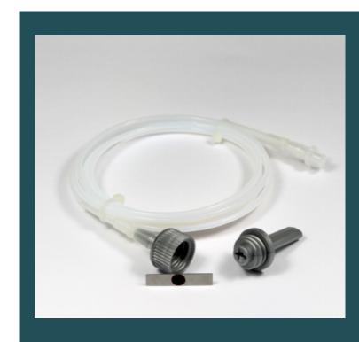
The ParaSure Single Lumen Channel Control 2 (SLCC2) simulates fine lumen devices and endoscope channels with a 2mm internal diameter, to effectively test the washer-disinfector's performance. The polypropylene head houses the indicator and is connected to a 1.5 metre length of PTFE tubing which terminates in a luer lock.
